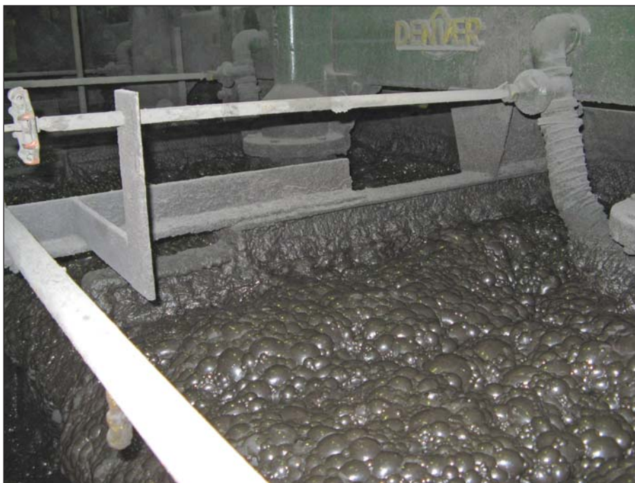
A zinc flotation circuit at the Scotia mine.
